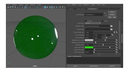
The material mimics the behavior of glass using two passes: The first pass is multiplicative and tints the background down by the glass color. This is similar to colored glass where only a part of the light / the color spectrum comes through. The second pass adds reflections.
